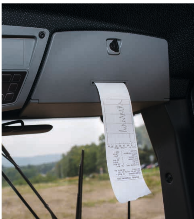
Integrated printer: for documentation of compaction results.
